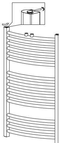
**Step 2:** Securely screw the heating element onto the radiator by spanner (clockwise).
